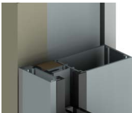
Figure 7: Curtain Wall Transition without Insulation between the Frame and Back-up Wall
