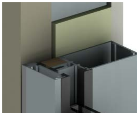
Figure 8: Curtain Wall Transition with Insulation
