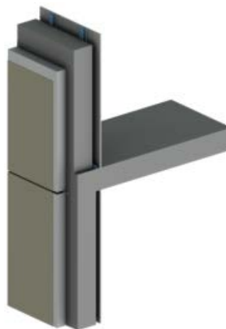
Figure 4: EIFS Concrete Wall Floor Slab Intersection
